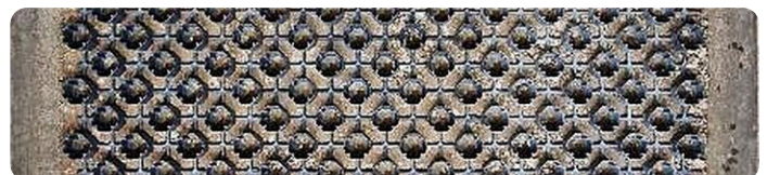
IIT Hyderabad: panels in the large-scale pavement test tank
